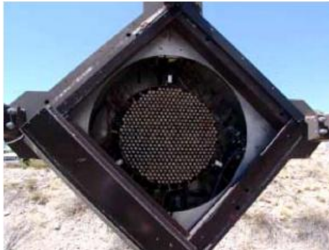
Figure 3-3 The T1 camera box with 499 pixel camera [1].
