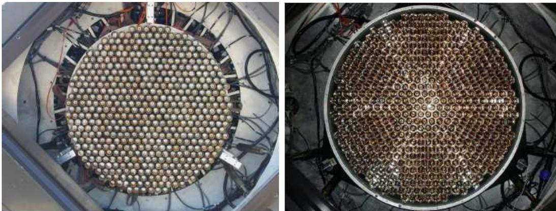
Figure 2.10: **(Left)** Frontal image of the camera without the light cones. **(Right)** Frontal image of the camera when the light cones are attached. Both taken from Cogan (2006).
