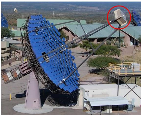
Figure 2.8: A VERITAS telescope. The red circle shows the box in which the camera is installed. Credit: Martin Schroedter/The VERITAS Collaboration.
