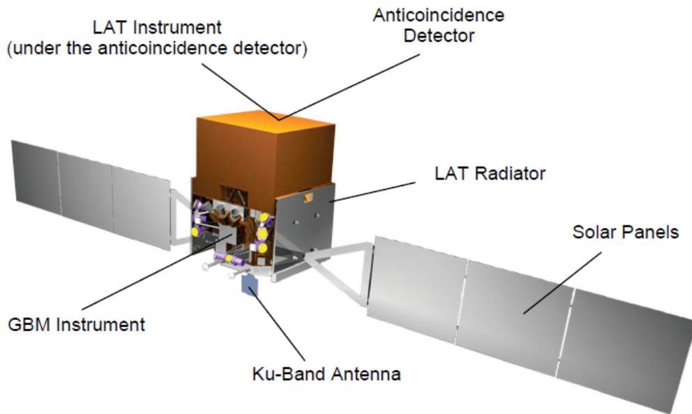
Figure 2.6: Fermi Gamma-ray Space Telescope. Images credit: NASA.
