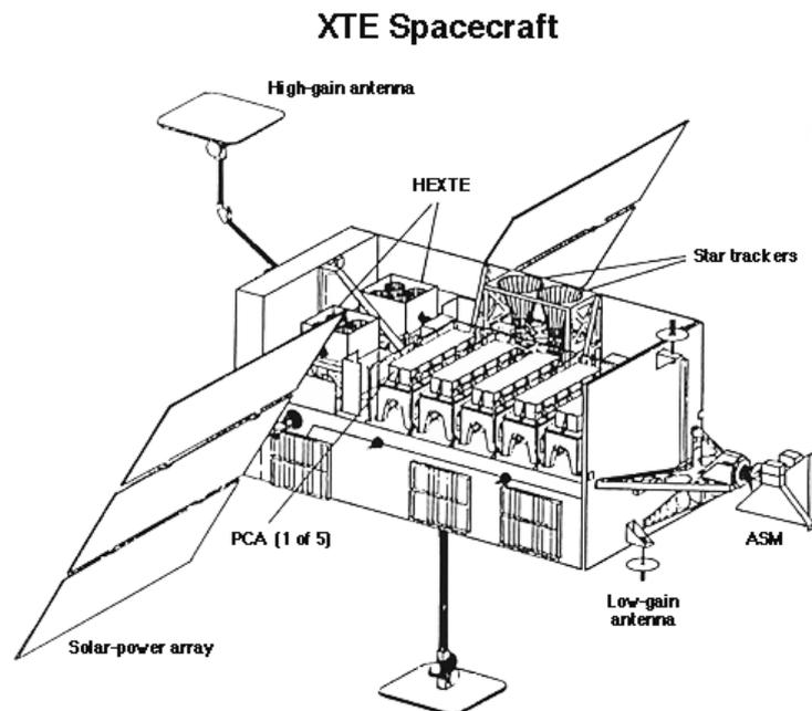
Figure 2.4: RXTE with the PCA, ASM and HEXTE. Courtesy of NASA.
