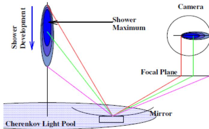
Figure 3.7: Schematic illustration of the imaging of an electromagnetic shower in the focal plane of an IACT located within the Cherenkov light pool. Image from Cogan (2006).
