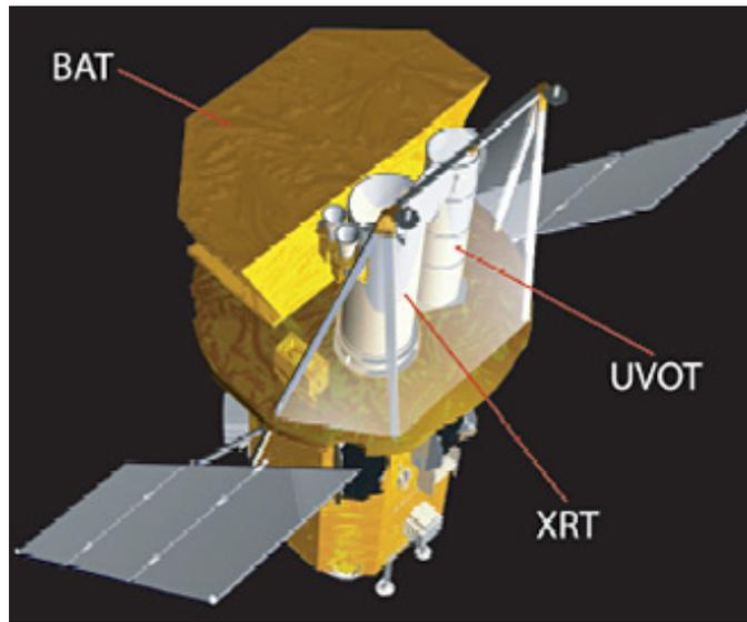
Figure 2.1: The Swift artistic impression with the three instruments. Drawing courtesy of NASA.
