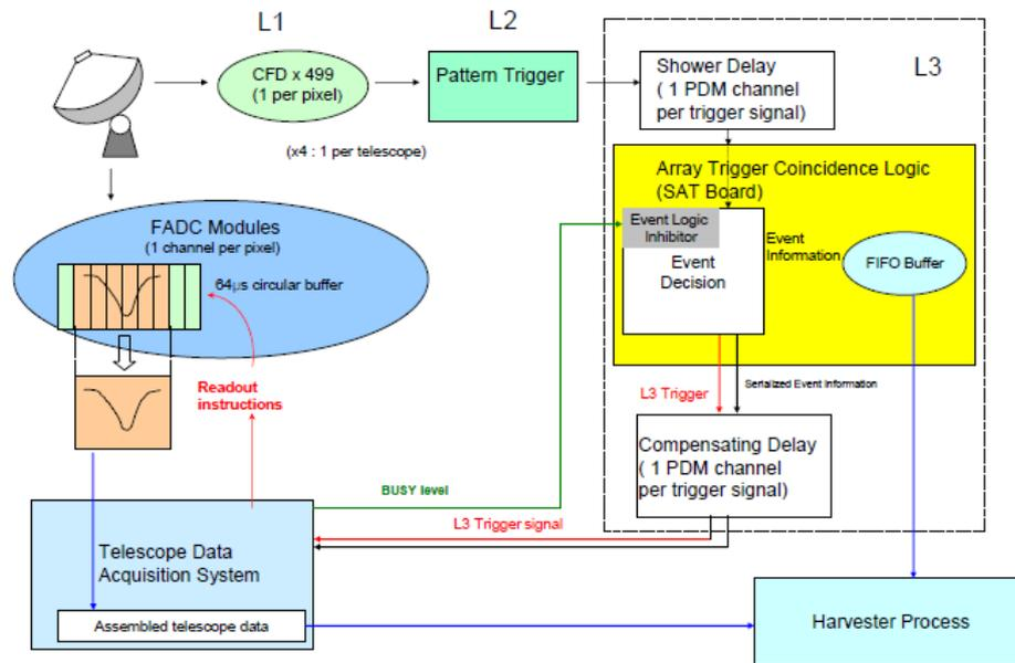
Figure 3.20: Schematic diagram of the VERITAS system trigger. Figure taken from (Weinstein 2007).
