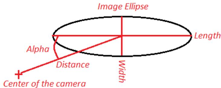
Figure 3.13: Hillas's parameters.
