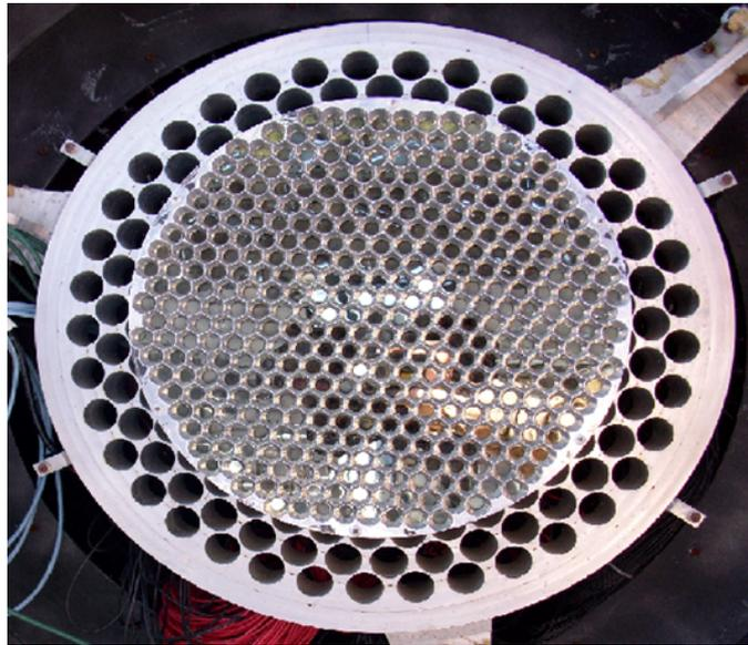
Figure 3.10: Camera of the Whipple 10m telescope.
