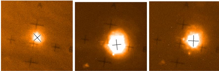
Figure 4.1: Bright star images at the focal plane of the Whipple 10m. The cross on the center of the four crosses (positions of the LEDs) is the center of the camera. *Left*: Polaris at  $31^\circ$  of elevation and  $0^\circ$  of azimuth. *Middle*: AlphaUma at  $60^\circ$  of elevation and  $358^\circ$  of azimuth. *Right*: DeltaLeo at  $78^\circ$  of elevation and  $206^\circ$  of azimuth.
