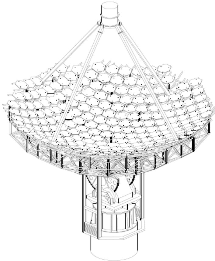
Figure 3.11: Structure of the Whipple 10 m telescope.
