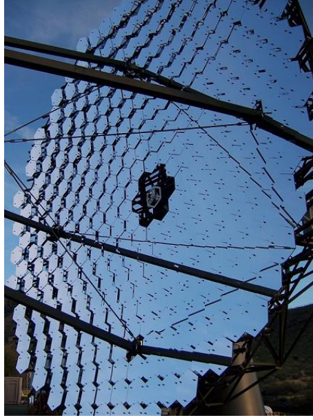
Figure 3.5: The VERITAS DC optical system with segmented mirror facets.
