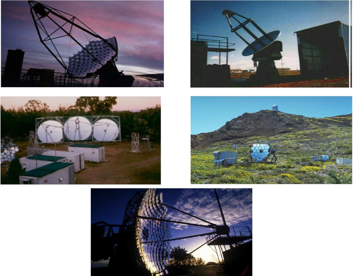
Figure 1.1: Photos of some of the second generation atmospheric Cherenkov telescopes. From left to right and top to bottom are shown *CAT*, *CANGAROO*, *Durham Mark 6*, *HEGRA*, and the Whipple 10m.
