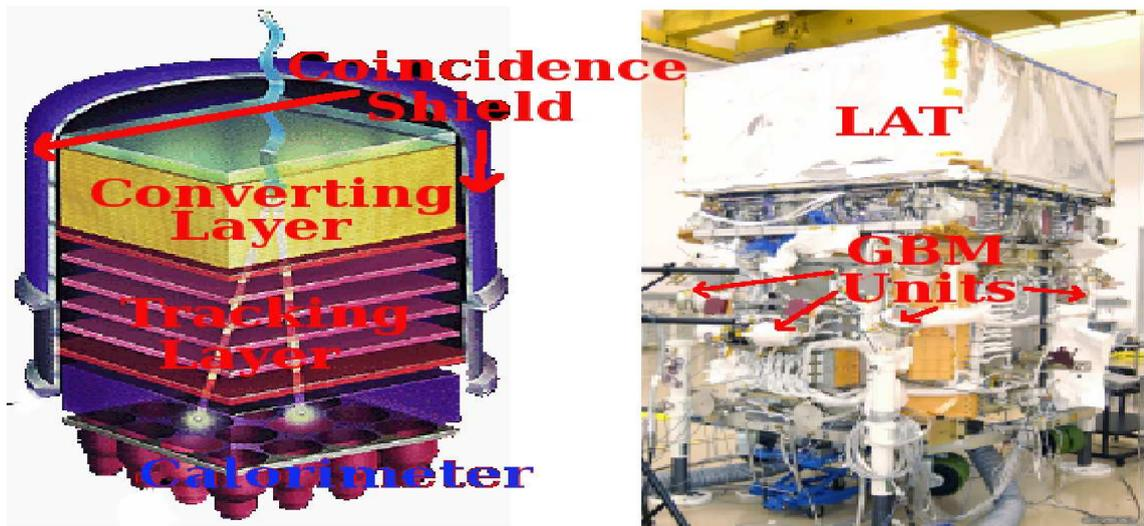
Figure 1.5: Left: The basic design of a pair-tracking telescope as it is explained in the text. Right: The GLAST satellite during environmental testing. It can be easily seen how the design on the left is integrated into the large section on the top (known as the *Large Area Telescope* or LAT). The locations of some of the *Gamma – Ray Burst Monitor* units are also shown- see section 1.1.5.
