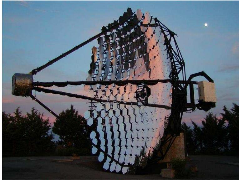
FIGURE 2.1. The Whipple 10 m telescope in its horizontal stow position.
