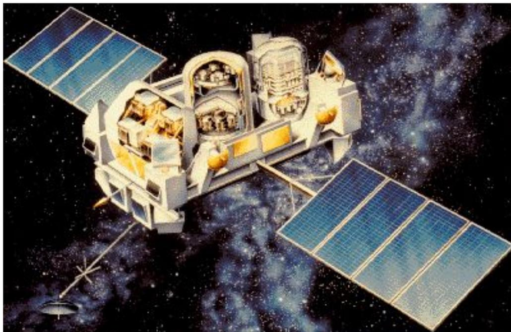
FIGURE 2.1: A collection of several instruments including EGRET (center) and BATSE (eight detectors, one on each corner of the spacecraft), the Compton Gamma Ray Observatory was highly successful in observing a wide range of  $\gamma$ -ray phenomena. Figure from <http://cossc.gsfc.nasa.gov>.
