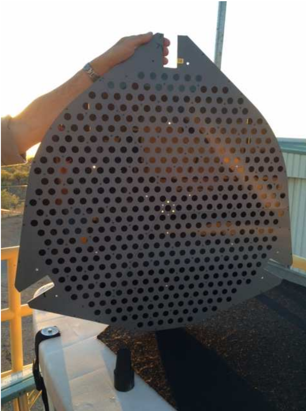
Figure 9.2: Picture of a UV filter plate. Each PMT has its own filter. The individual filters are larger than the exit aperture of the light cones. The bright points near the center of the image are daylight coming through the filter assemblies. Image credit: D. Hanna.
