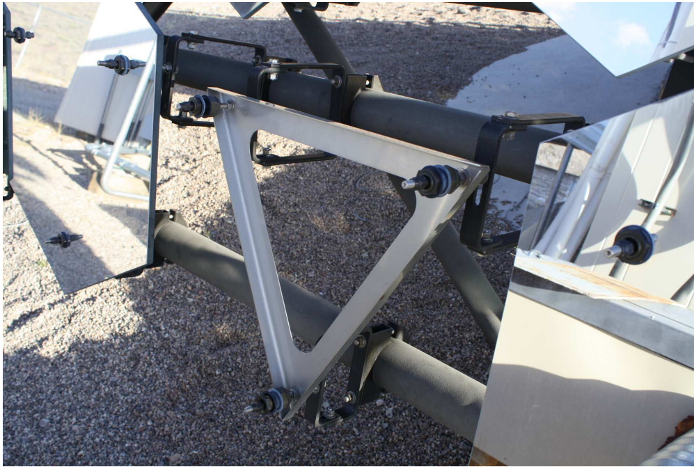
Figure 3.14: A VERITAS mirror mount. Each of the three points of the mount is a combination of a mounting bolt (so the mirror facet can be fixed to the mount) and a fine-alignment screw connected to a gimbal which allows for the facet to be adjusted.
