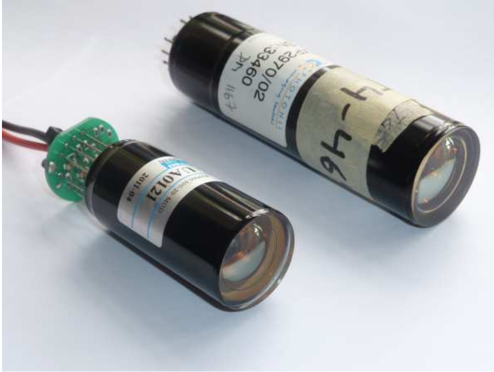
Figure 3.9: Front: Hamamatsu R10560-100-20 MOD PMT used since September 2012. Back: Photonis XP 2970/02 PMT used on VERITAS prior to the upgrade. Image credit: Figure 1 in [42].
