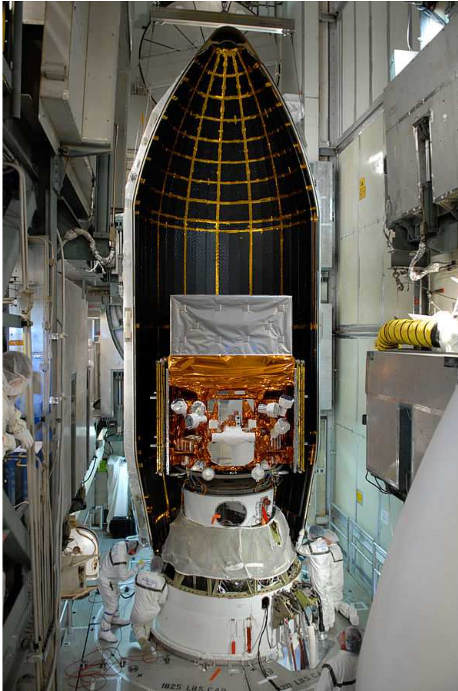
Figure 2.11: The Fermi satellite in its launch fairing in 2008. The LAT is the large silver “box” in the centre of the picture; the cylindrical GBM instruments can also be seen below it. Image credit: “First half of the payload fairing is installed around GLAST” by NASA/Jim Grossmann - Licensed under Public Domain via Wikimedia Commons
