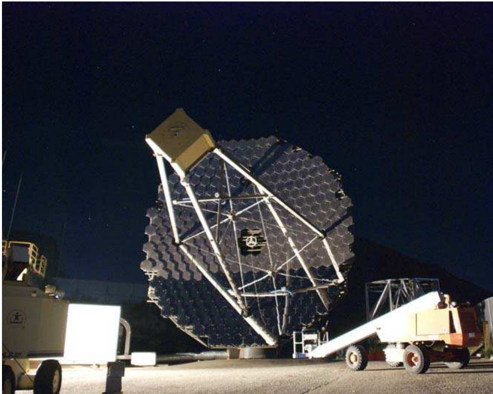
Figure 3.15: VERITAS Telescope 2 after a fresh batch of mirrors were installed on the bottom third of the dish. They appear to be darker because they are not coated with dust and small scratches due to being exposed to the elements, so there is less diffuse reflection. Image credit: VERITAS collaboration.
