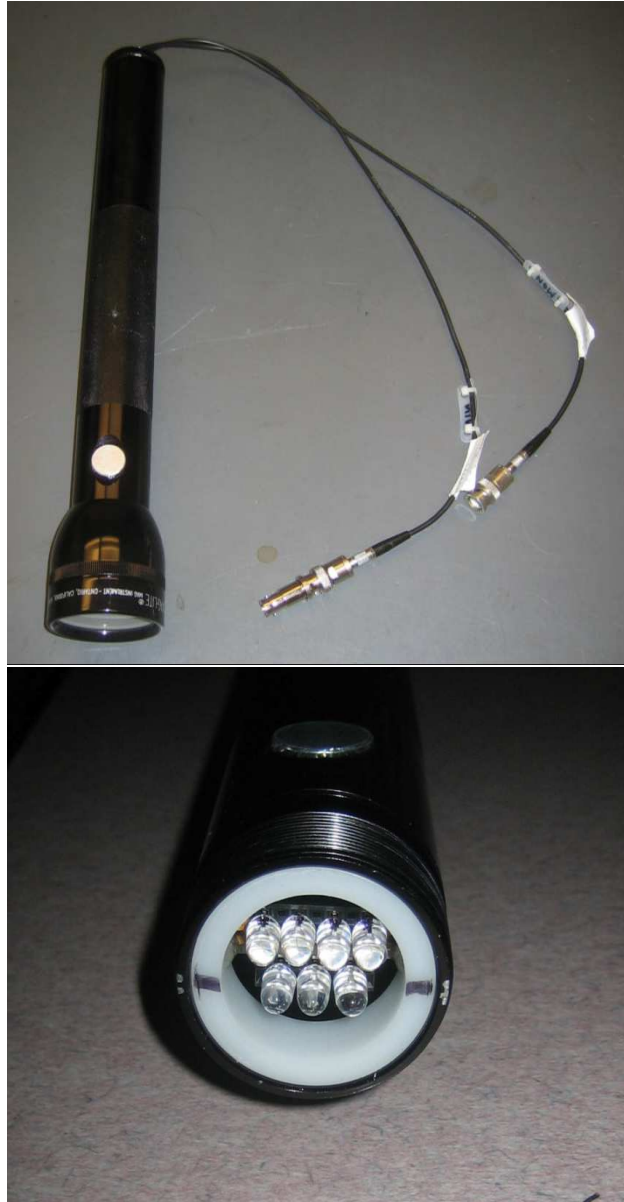
Figure 3.20: Top: An LED flasher. One is permanently installed on each telescope \sim 4 m from the camera. Bottom: Underneath a diffuser (not shown here), the 7 LEDs can be seen. Image credit: Figure 1 in [53].
