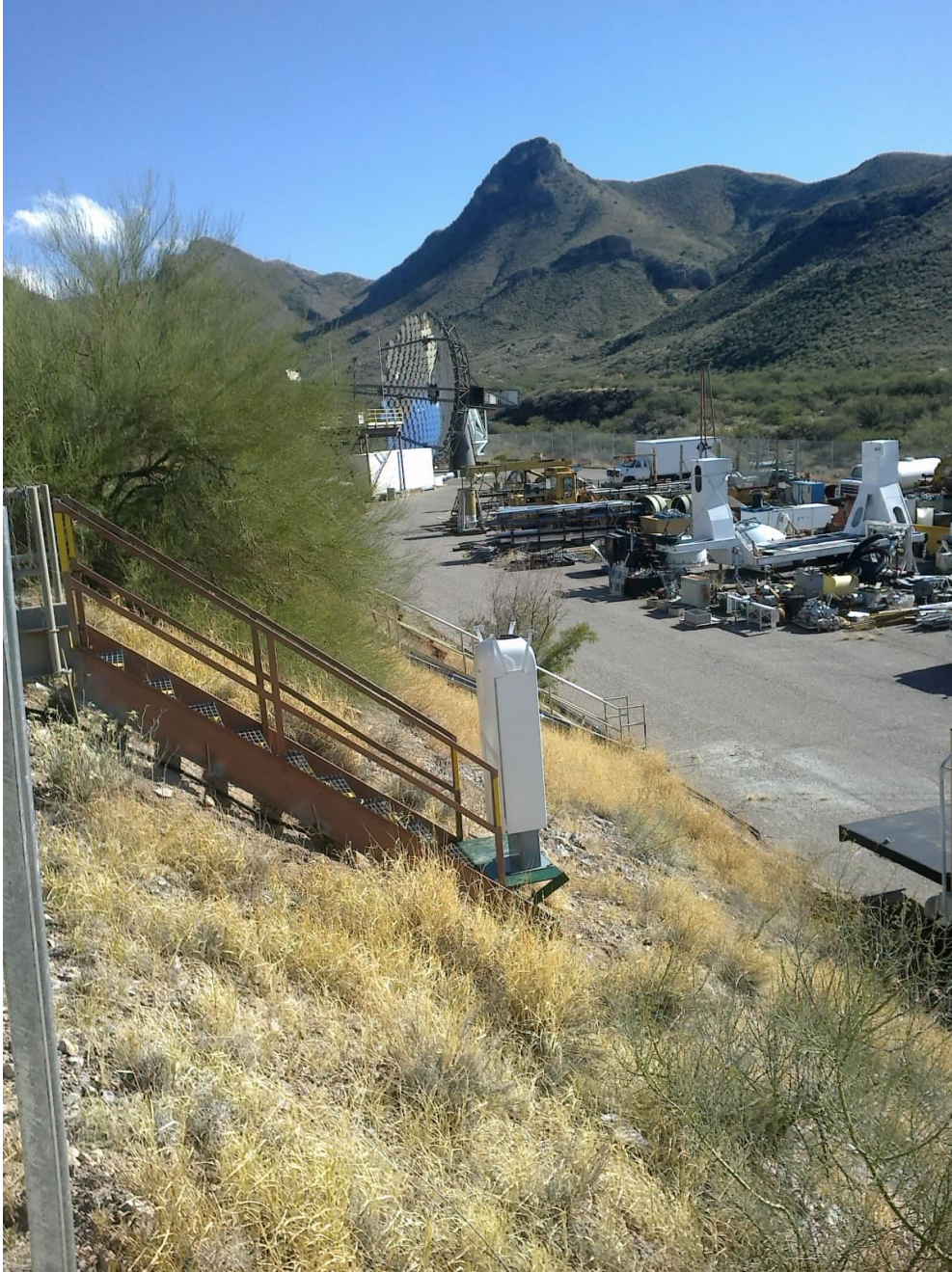
Fig. 4.1 A photograph showing the positioning of the ceilometer at FLWO. It sits \sim 3 metres above the base of Telescope 2 seen in the background, and \sim 1 -3 metres below Telescopes 1, 3 and 4. (Picture: J. Reynolds)
