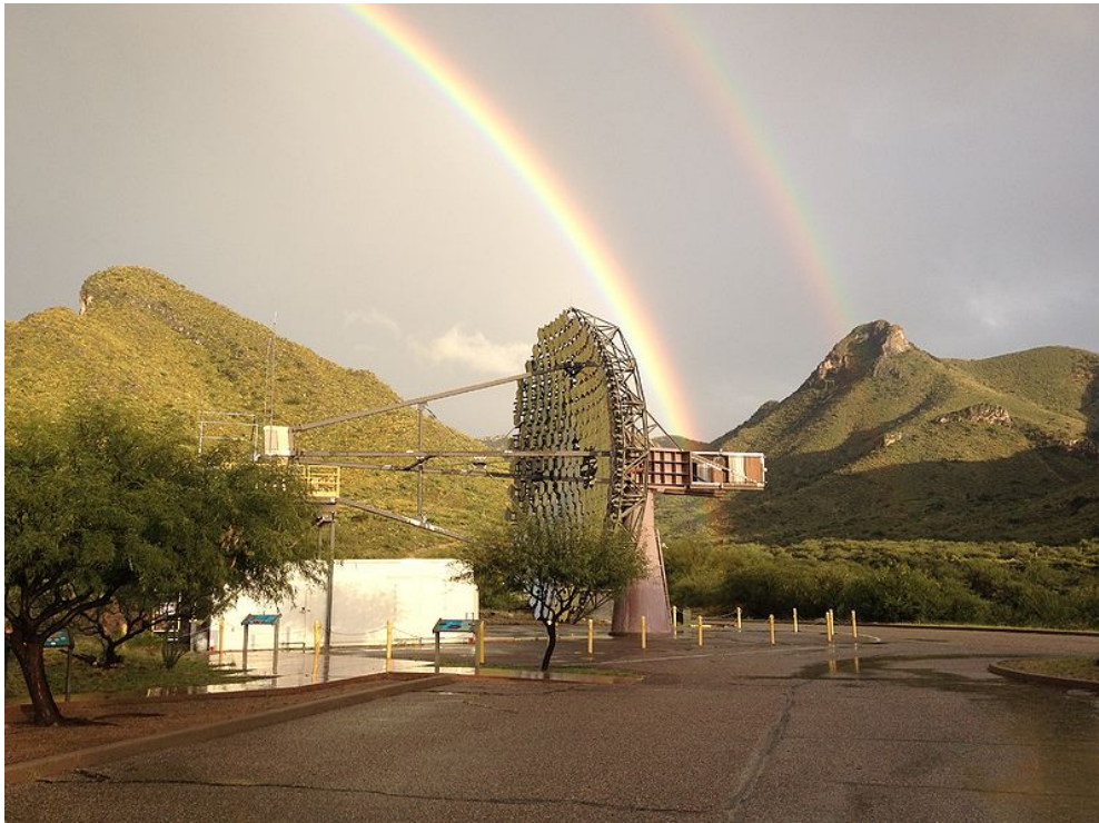
Fig. 3.6 A photograph of VERITAS Telescope 1, post 2009 move, showing the electronics trailer and a side view of the optical support structure, with a camera box at the focal plane. The tessellated mirrors are visible edge on.
