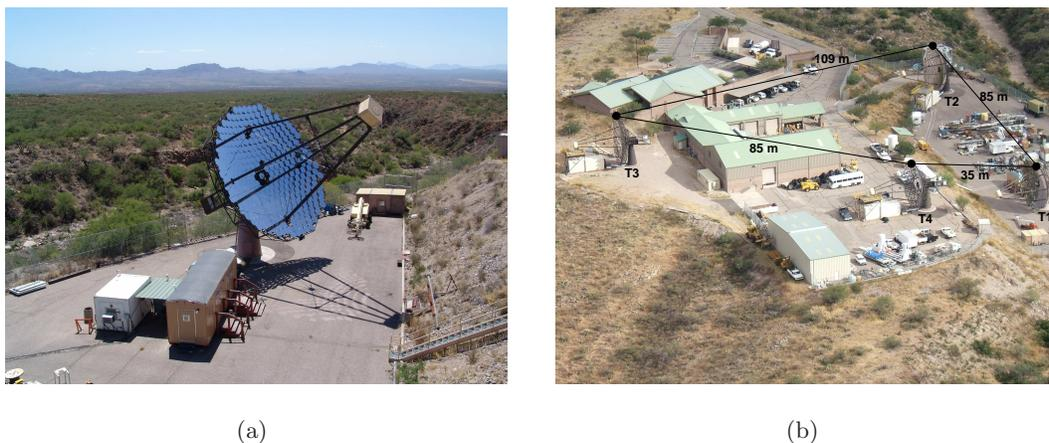
Figure 3.1: (a) The first VERITAS Telescope installed at the Whipple Observatory base camp. The control room housing the electronics and power supply systems is shown in the foreground. (b) The full VERITAS four telescope array from the air with the telescope separations marked.
