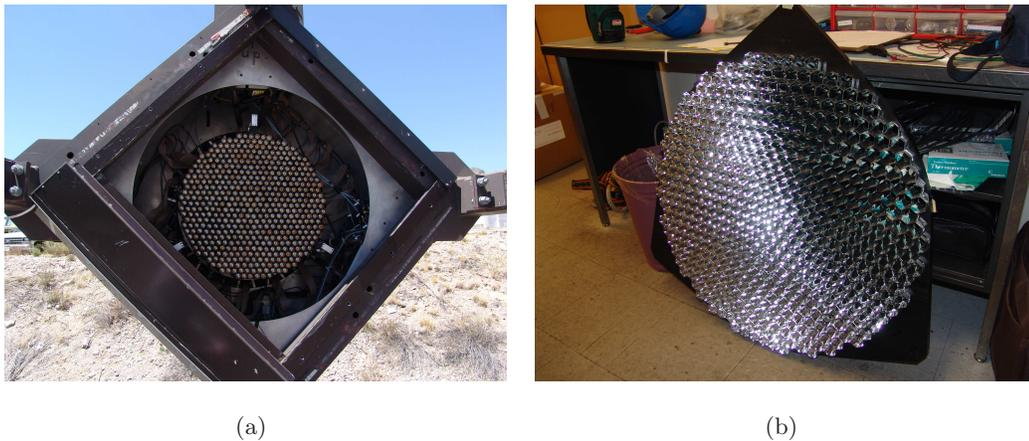
Figure 3.5: (a) The 499 PMT pixel camera. The focus box is 1.8 m square. A remotely operated shutter usually covers the camera during daylight hours. (b) The light cones set into a plate which in turn attaches to the camera.
