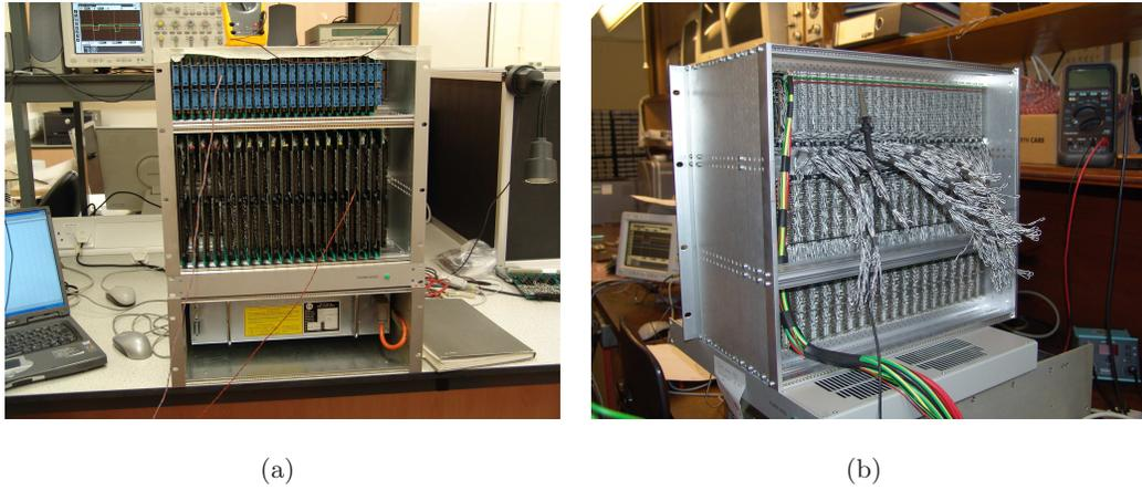
Figure 3.9: *The front, (a), and rear, (b), of the SS crate showing the intricate wire-wrapping on the backplane.*
