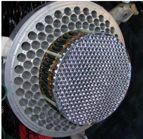
**Figure 4.6:** The 379-pixel high-resolution PMT camera of the Whipple 10 m telescope. Light cones are mounted in front of the PMTs to collect light that would otherwise fall in the gaps between the pixels.
